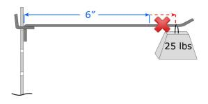
If the 25 lbs load moves further away than 6" from the pegboard face, the slatwall could break
