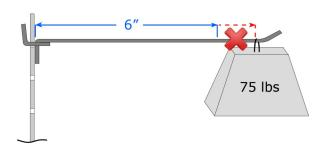
If the 75 lbs load moves further away than 6" from the pegboard face, the pegboard could break
