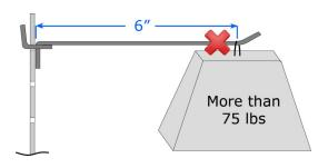
If the load increases to more than 75 lbs, the pegboard could break
