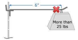
If the load increases to more than 25 lbs, the pegboard could break
