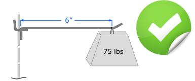
PegBoard  $PX^{TM}$  can hold a 75 lbs point load hanging at a 6" distance from the pegboard face:
