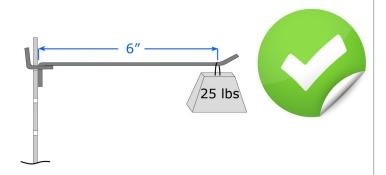
PegBoard  $PX^{\text{TM}}$  can hold a 25 lbs point load hanging at a 6" distance from the pegboard face:
